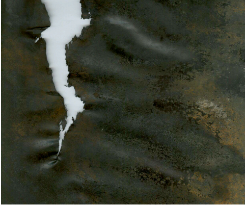
Figure 1. Photograph of a chemically attacked geomembrane. Note loss of ductility and thinning. The polymer became sticky and perished (courtesy of ExcelPlas Geomembrane Testing).
